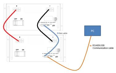
Note: RS485 communication address can not be 0, the address set by the host computer is required to be the same as the battery communication address, do not have duplicate addresses, otherwise communication may be affected.
