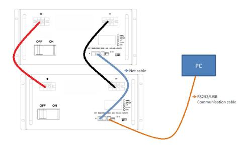
Note: In RS232 communication, any address bit can be used in single computer communication. In parallel communication, the host address must be 1, do not have duplicate addresses, otherwise communication may be affected.
